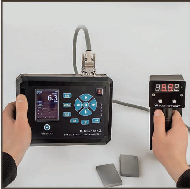
In addition, the device is used for testing the surface layers of ferromagnetic materials and the metal for presorting steel grades.
