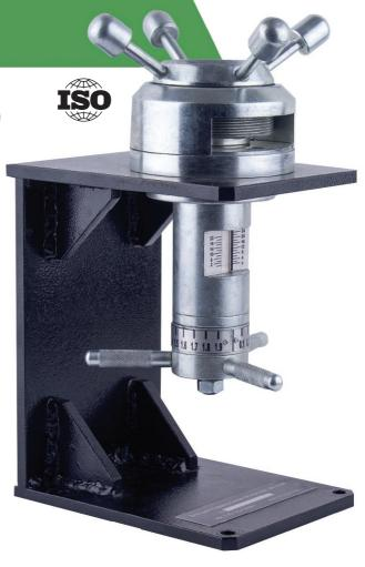
The Ericksen's device is used for determining the strength of the coating at the indentation of spherical tip punch with diameter of 20 mm in the coating of the sample, the position of which is fixed on a matrix with internal diameter of 27 mm.
