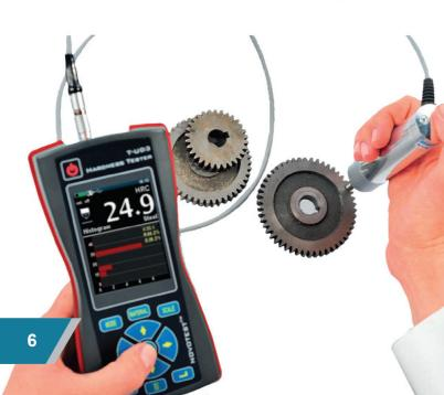
The using of diamond indenter allows setting the probe precisely in any tiny point. The depth of the imprint left by Hardness tester T-U3 is many times smaller than imprint left by standard Rockwell hardness tester, which makes this method of measuring the least destructive.
