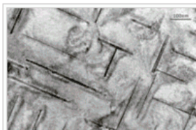
Aluminium copper (4 at% Cu) alloy showing copper precipitation within the aluminium matrix. The image is a projection through the metal where the dark regions are plate like copper precipitates
