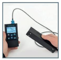
Concrete Cover Meter NOVOTEST Rebar Detector works in a mode of constant scanning of the test
