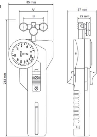
\*The measuring head width is depending on the outer distance between the outside guide rollers
