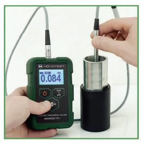
Coating thickness gauge is a precision measuring instrument for rapid non-destructive testing of coatings in accordance with standard **ISO 2808.**
