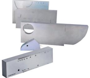
Calibration blocks are used to configure the sensitivity and duration of scan of ultrasonic flaw detectors during testing of various products (mainly flat sheets and pipes).
