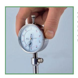
It is used for (depending on configuration): measures the peak-to-valley height of a blast cleaned surface; measurement the depth of focal corrosion; measures depth of narrow holes and grooves.
