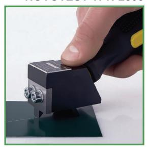
Paint inspection gauge TPN-2808 is designed according to ISO 2808, ASTM B 4138, DIN EN 1071-2 to measure the thickness of both single and multiple layer coatings on any grounds, both metallic and non-metallic.
