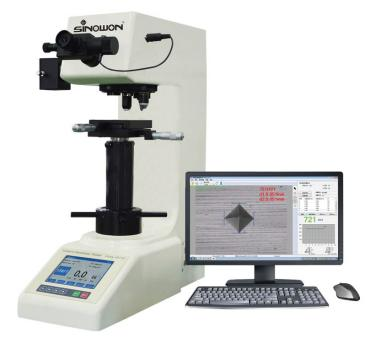
Sinowon new generation vickers/knoop measurement software with friendly operation interface, apply USB camera to fast capture video and images, supports case depth inspection by analyzing the indentation image.
