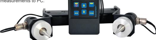
Also it has: mode of the signal visualization (A-scan), the ability of testing concrete (and other) constructions for internal defects and discontinuities, also increases the accuracy of measuring time intervals by manual timing of the moment activation of measurer.
