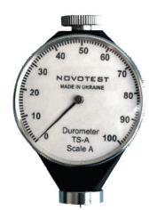
Shore Durometer NOVOTEST standardized according to ISO-7619 and ISO-868, DIN53505, ASTM D2240 and JIS K7215.
