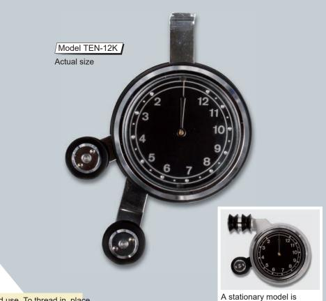
The instrument is designed for one-hand use. To thread in, place the yarn between the two guide rollers. Push and hold the key button at the instrument. The outer roller will be turned up and the instrument is ready for measuring. The measured value will be displayed at the analog display.
