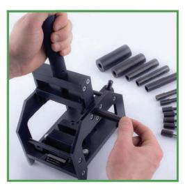
The device complies with **ISO 1519-73**, **DIN 53 152** and applies to paints and specifies a method for determining the elasticity of the film by bending.
