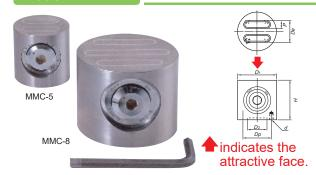
These chucks are used in combination with a magnetic chuck as an auxiliary holding tool for irregularly shaped workpieces in grinding and light duty cutting. (These chucks cannot be used in wet operations.) They can also be used for such applications as holding workpieces in advance to reduce the setup time. Thus they can be used for continuous grinding of small and thin workpieces
