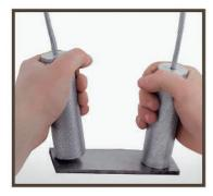
Magnetic flaw detector is based on the method of non-destructive testing used for detecting violations of the magnetic surface of metal structures and structures of ferromagnetic materials.
